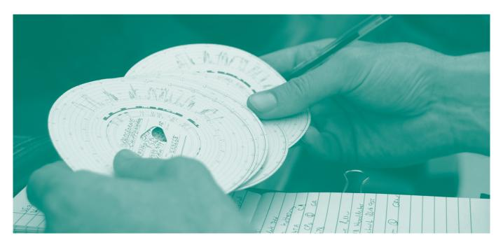
An approved tachograph is the required instrument by which the activities of drivers subject to the EU or AETR drivers' hours rules, and the vehicle's speed, distance and time are recorded. There are two main types of tachograph – analogue and digital. The only exception is when driving a vehicle engaged in the collecting of sea coal. In this one case you are subject to the EU rules on drivers' hours but do not need a tachograph.
