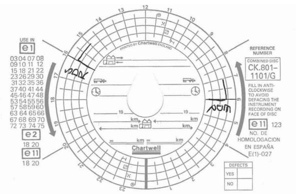
This is an example of manual entries made on the rear of a tachograph chart of a driver who started his day at 06.00 with an hour's work doing other duties away from his vehicle. He also finished his day with an hour of other work away from his vehicle and has indicated both the end and the start of a daily rest period. His activities while with the vehicle are recorded by the instrument on the other side of the chart once it has been inserted.
